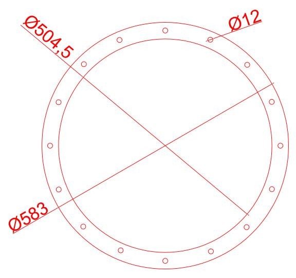
500 Diameter flat bar flange 5mm thick 16 x 12mm holes PCD 549mm Weight 2.67 Kg Electro plated
