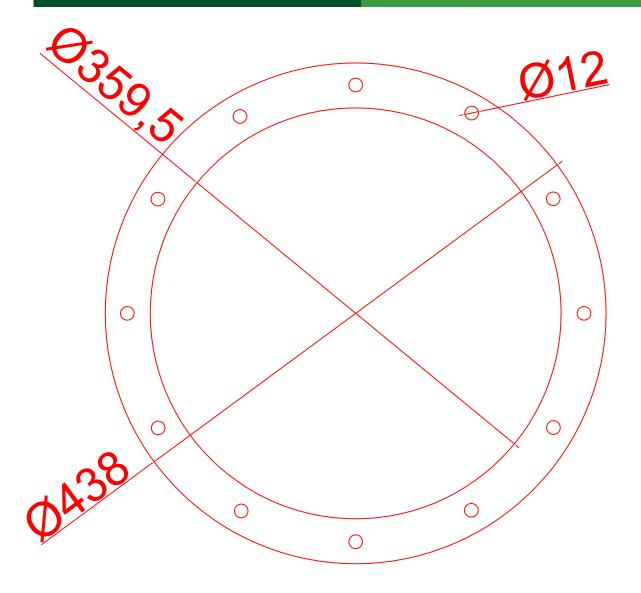
355 Diameter flat bar flange 5mm thick 12 x 12mm holes PCD 403mm Weight 1.96 Kg Electro plated
