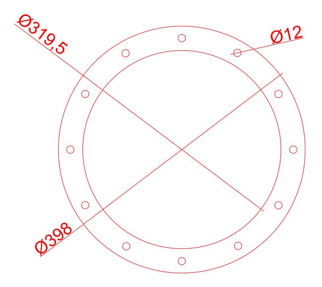
315Diameter flat bar flange 5mm thick 12 x 12mm holes PCD 362mm Weight 1.76 Kg Electro plated
