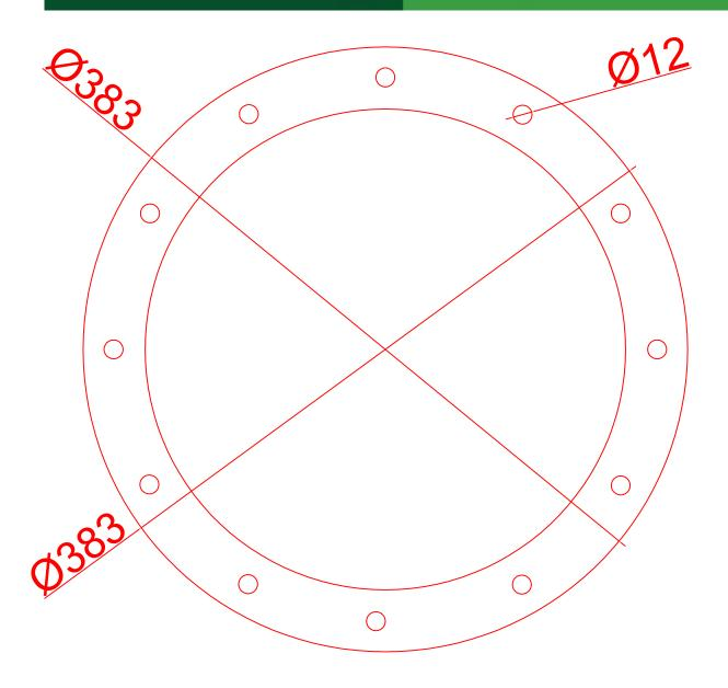
300 Diameter flat bar flange 5mm thick 12 x 12mm holes PCD 352mm Weight 1.69 Kg Electro plated
