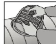
Turn the knobs till they hit the stops and insert the inner door panel inside the opening at an angle. Then straighten the door, pull it lightly to center it and tighten the knobs.
