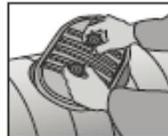
Turn the knobs till they hit the stops and insert the inner door panel inside the opening at an angle. Then straighten the door, pull it lightly to center it and tighten the knobs.
