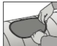
Both ends should meet at a straight section of the opening. Cut the SKK at the right length so that both ends press slightly against one another without overlapping.
