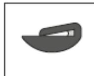
The SKK molding is fitted with injected glue. It can be applied on duct walls up to 2 mm thick (Gage ≈14)
