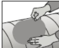
Apply the self-adhesive template on the duct wall at the desired position.
