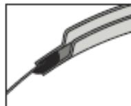
The thicker lip of the SKK must be inside the duct. Apply the SKK molding so that the duct wall enters as deeply as possible into its pocket.
