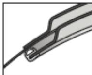
Place the silicon ring around the edge of the inner access door panel, making sure that the thicker side is between the two access door panels.
