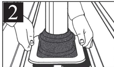
2 Slide Dektite® flashing down over pipe. Water can be used as a lubricant
